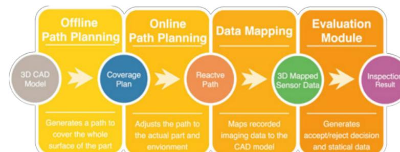
All the components are designed to be “general” methods which can deal with different camera models (RGB-D, Infrared, and X-ray) so that the system can be configured for any kind of imaging sensor suitable for any inspection task.
